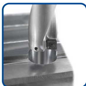
Stegbohren Rack drilling
