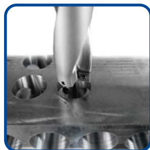
Vollbohren Solid drilling
