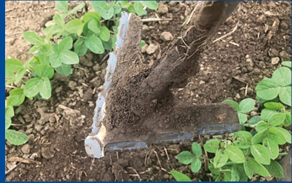
HS160A2, after approx. 100 ha, saw teeth still clearly visible
