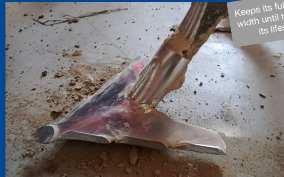
HS160A1 after 600 ha on 12-row cultivator, 15 - 20% of the max. life time still remaining
