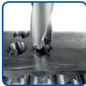
Düz delik Solid drilling
